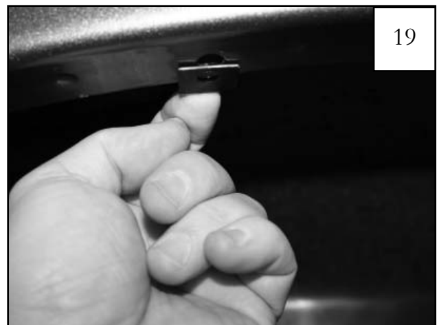
Install Clip (CL1-0022) over existing hole.
