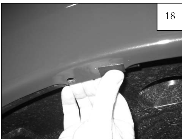
Install plastic tab over existing factory hole.
