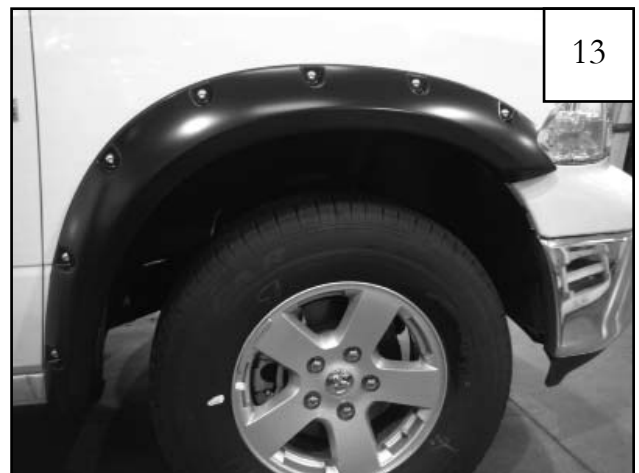
Completed front flare installation.
